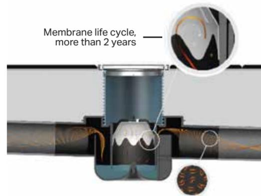
Water seal lasts 5 times more, thanks to the reduced evaporation rate.
